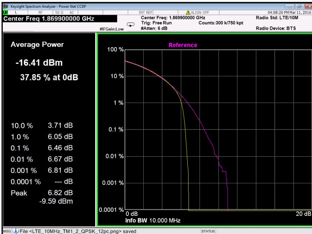
**Figure 2: CCDF for 10 MHz LTE, TM1.2 with 12% EVM.**
