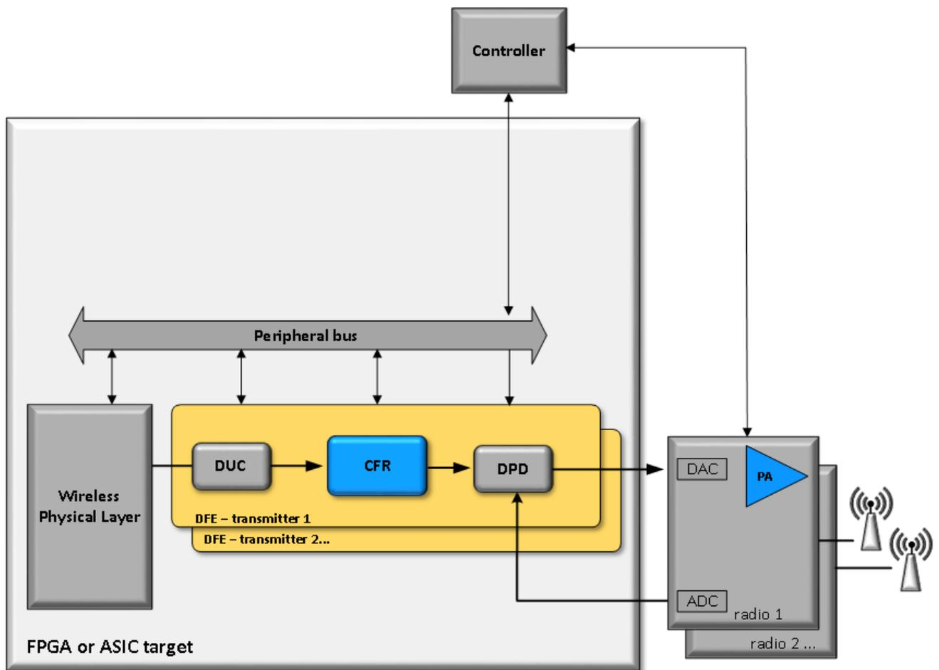
Figure 1: FlexCFR example sub-system architecture.
