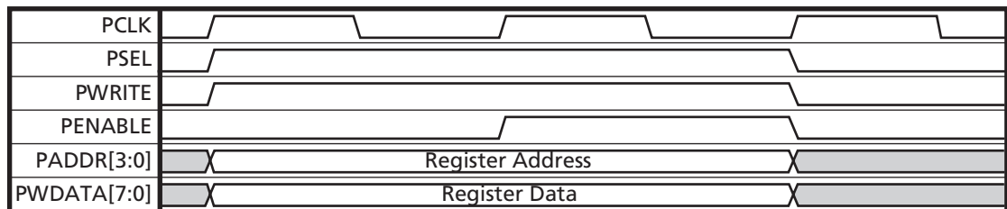
Figure 3-2 · APB Data Write Cycle
