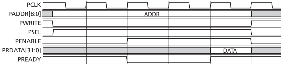
Figure 5-1 · APB Interface Control/Status Register Read Cycle
