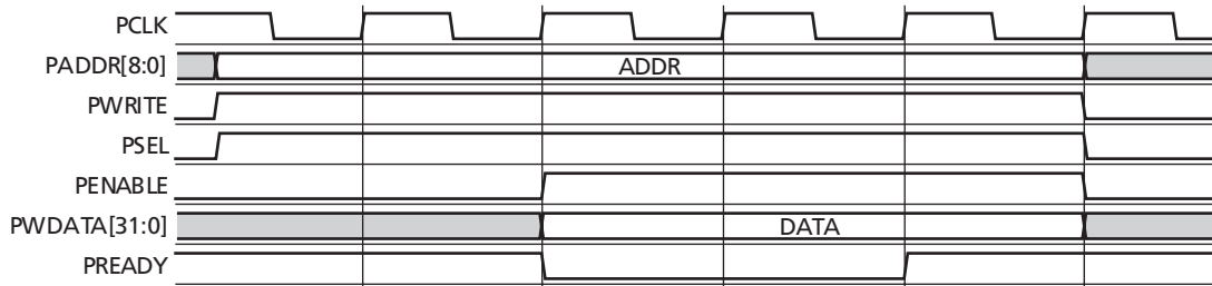
Figure 5-4 · APB Interface Data Register Write Cycle
