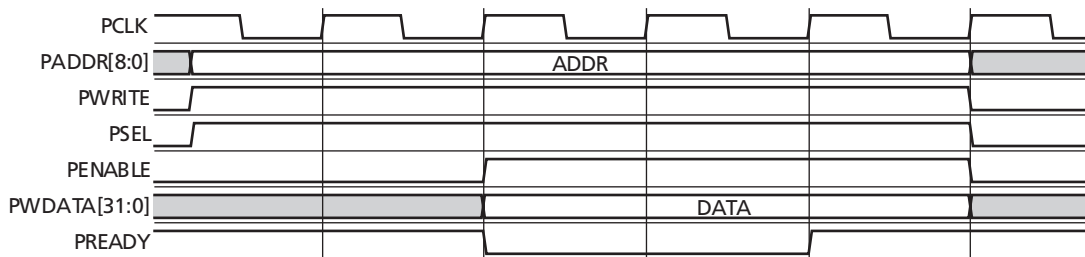
Figure 5-6 · APB Interface Label Memory Write Cycle
