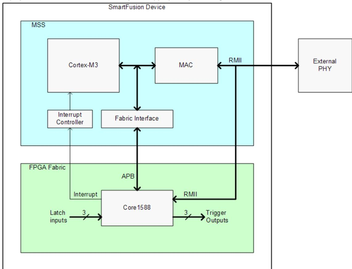
**Figure 1** Core1588 in a SmartFusion Device
