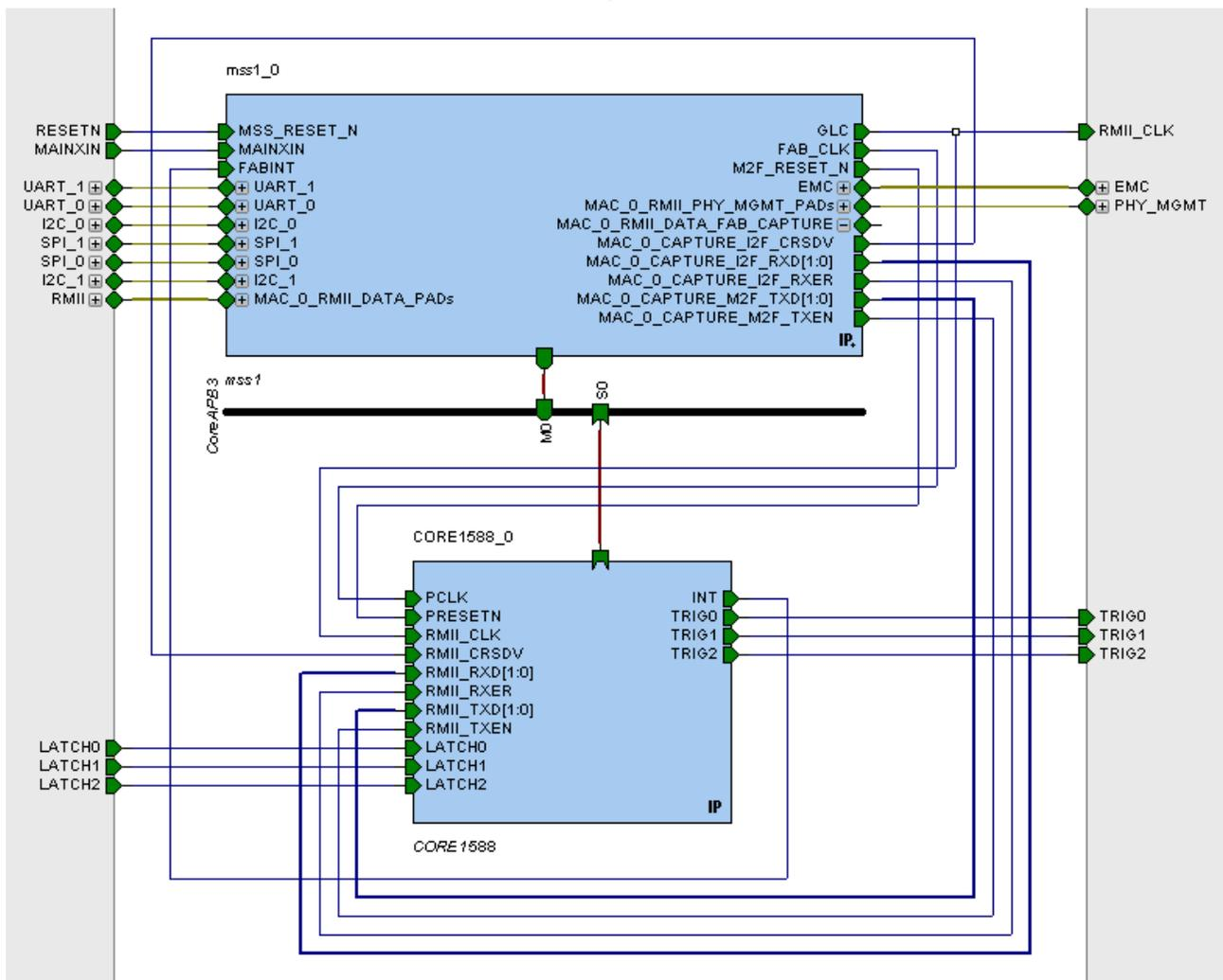
**Figure 7** Core1588 System Example
