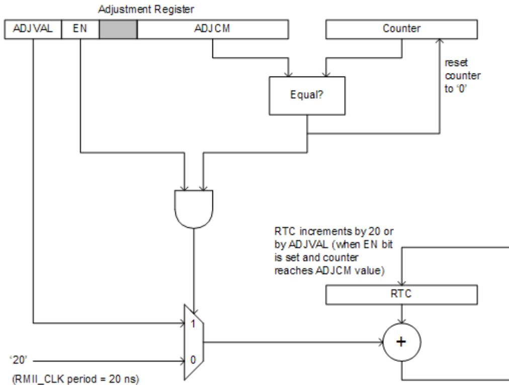
Figure 3 Role of the ADJUST Register in Controlling RTC Rate
