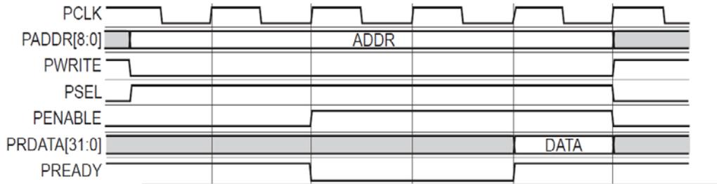
**Figure 8** APB Interface Control/Status Register Read Cycle
