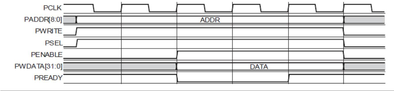
**Figure 13** APB Interface Label Memory Write Cycle
