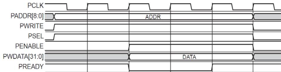
**Figure 9** APB Interface Control Register Write Cycle
